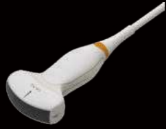
1 - 5 MHz Single Crystal Curved Array
